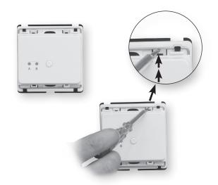
**3**: Mount the backing plate in the wall socket using a screwdriver and screws supplied.
