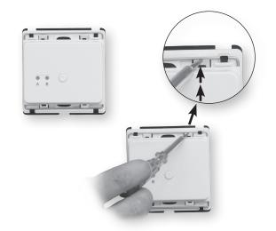
**3**: Mount the backing plate in the wall socket using a screwdriver and screws supplied.
