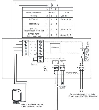
Boiler / zone valve switch Voltage free OR with link 230V
