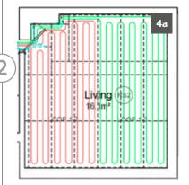
Before attempting to lay any floor heating boards, familiarise yourself with the system layout drawing, noting manifold position. The drawing will detail the orientation and position of panels (4a).
