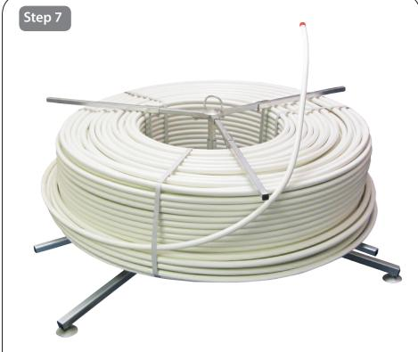
Top arm carrier **A** and top arms **D** can now be removed as one section. Pipe is installed centrally over main body **B** and sat onto lower arms **E**. Replace top arm carrier **A** and top arms **D**, the height adjustment bolt on main body **B** can now be tightened and top arm stops **C** adjusted to suit size of pipe coil. Ensure bolts are tightened and secure.
