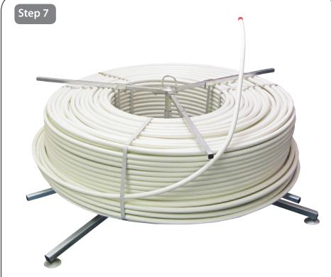
Top arm carrier  $\bf A$  and top arms  $\bf D$  can now be removed as one section. Pipe is installed centrally over main body  $\bf B$  and sat onto lower arms  $\bf E$ . Replace top arm carrier  $\bf A$  and top arms  $\bf D$ , the height adjustment bolt on main body  $\bf B$  can now be tightened and top arm stops  $\bf C$  adjusted to suit size of pipe coil. Ensure bolts are tightened and secure.
