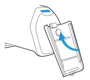
Remove the battery cover 3 from the top of the Smart Radiator Head.
