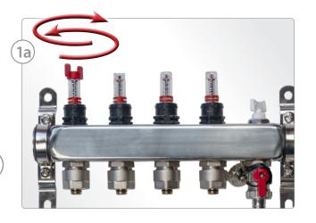
IMPORTANT: Adjust by hand only and do not force beyond two full turns from shut as this may cause damage to the flow meter.
