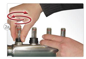
IMPORTANT: Adjust by hand only and do not force beyond two full turns from shut as this may cause damage to the flow meter.
