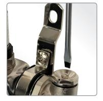
Re-open all return valves. And open the air vent on the return bar, close when all air has been vented. Allow the pressure to rise to 3-4 bar, (pic K) close the red tap on the flow bar (pic L). Turn off the mains water supply hose at source and leave the system under pressure for a minimum of 3 hours.
