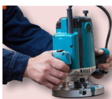
Router with suitable routing bit (pipe diameter 16/12mm) for cutting extra channels.
