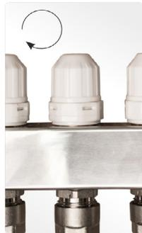
This will ensure that any air introduced from the feeds to the manifold can be vented using the manual air vents not allowing any air into the UFH loops.
